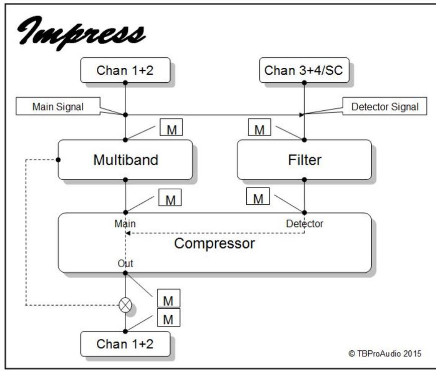
**Compressor:** The compressor part has two inputs (Main and Detector) and one output (Out): the main signal is the audio stream to be processed by the compressor, the detector signal is the signal for the level detection. In most applications both signals are the same, for side-chain effects separate signals are used.
