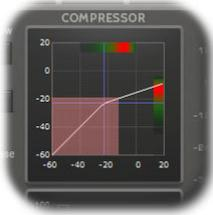
This display shows the current gain transfer curve (white line), current threshold value (blue line), maximum main signal level (red area) and current main signal level (light red area). Additionally heat-maps of main signal (top) and output signal (right) are shown.
